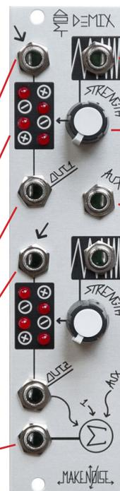
**CARRIER CV IN:** Determines amplitude & phase of Channel 1 Signal In.
