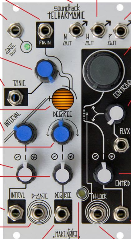
**CENTROID ROTARY:** This rotary has a different effect on the output: **H Out** - modulates or selects harmonics for emphasis by **Flux** and **H-Lock** parameters. **P Out** - sets the phase modulation ratio. **N Out** - No effect.
