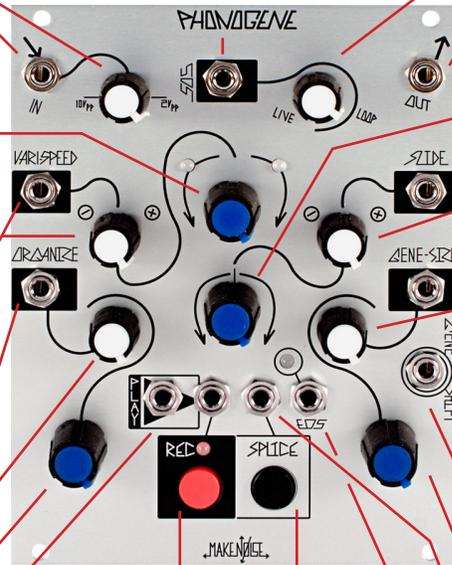
**SLIDE ROTARY:** Manual bipolar rotary for scanning the pieces of sound that result from setting Gene-Size to greater than 10%. Moves/slides through the Genes (aka grains). Allows for scrubbing of the recorded material, and is always dependent upon the Gene-size setting.
